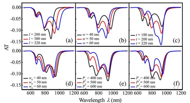
**Fig. 5.** Asymmetric transmission (AT) spectra of OIN arrays in the gold film with different (a) length  $l$  values, (b) width  $w$  values, (c) thickness  $t$  values, (d) width  $w_0$  values, (e) period  $P_x$  values, and (f) period  $P_y$  values.
