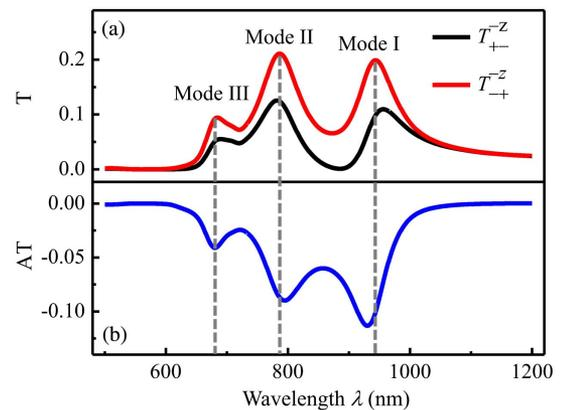
**Fig. 2.** (a) Transmission spectra of OIN arrays in the gold film under circularly polarized excitation along  $-z$  direction. (b) AT spectrum of OIN arrays in the gold film. The three resonances are labeled modes I, II, and III.
