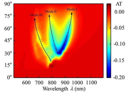
**Fig. 4.** Color map of AT values of OIN arrays in the gold film with angle  $\beta$  changed from  $0^\circ$  to  $90^\circ$ .
