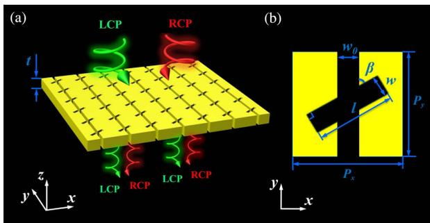
**Fig. 1.** (a) Schematic of OIN arrays in the gold film with  $P_x = P_y = 500$  nm,  $t = 200$  nm,  $w = 50$  nm,  $w_0 = 50$  nm,  $l = 300$  nm, and  $\beta = 60^\circ$ . (b) Its unit cell with the associated parameters definition.
